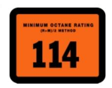
Rockett Brand 114 Racing Gasoline is a very high octane, high quality leaded fuel designed exclusively for racing applications at sanctioned racing events. It has an octane rating (AKI) of 114 and a Motor Octane Number of 110. It is specially formulated for high compression engines, both small blocks and big blocks.
